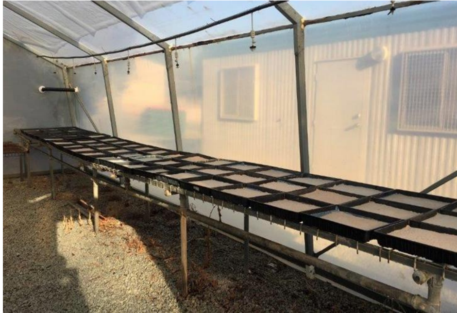
Plate 12: Seed trays in GA hot house undergoing rapid ageing wet/dry cycles, April 2017
