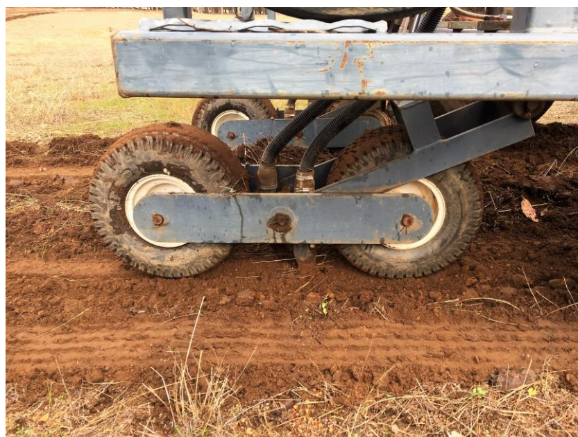
Plate 31: Configuration of CommVeg seeding arms featuring forward press wheel, seed openers and a trailing press wheel
