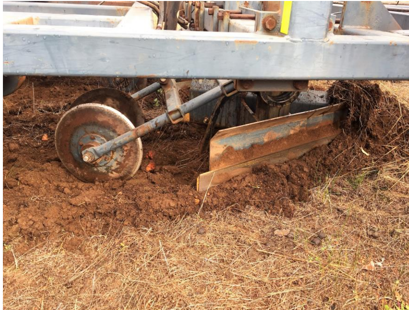
Plate 30: Configuration of mini scalp, ripping tyne and plough disc on CommVeg seeder
