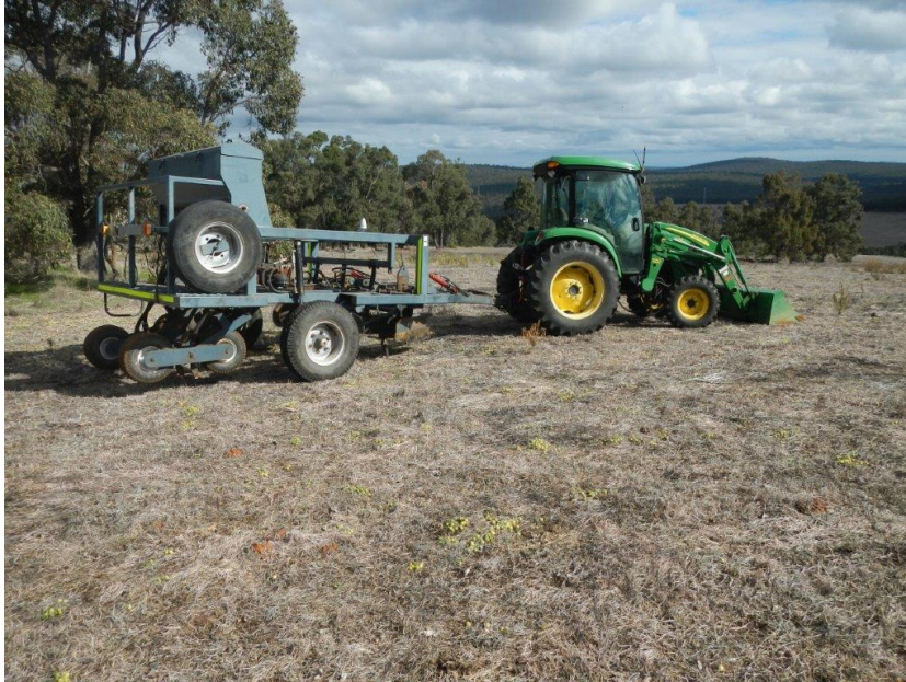
Plate 29: Commercial native vegetation seeder (CommVeg Seeder) and tractor configuration used at Hotham Farm
