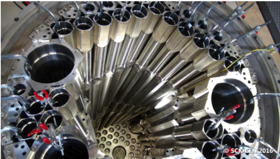
Beryllium reflector rods made by Materion shine through the center of the partly assembled mock-up for the BR2 matrix refurbishment. Photo provided by SCK-CEN.
