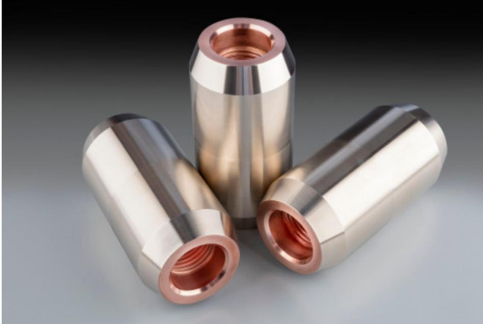
The new VRGB coupling, which connects the rod string to the pump drive rod, restricts the valve rod bushing from coming in direct contact with production tubing due to its thick-bodied design. ToughMet material is a low friction alloy, and therefore preserves adjacent production tubing and minimizes the risk of tubing leaks. In addition, the coupling can withstand high impact loads from rod buckling.
