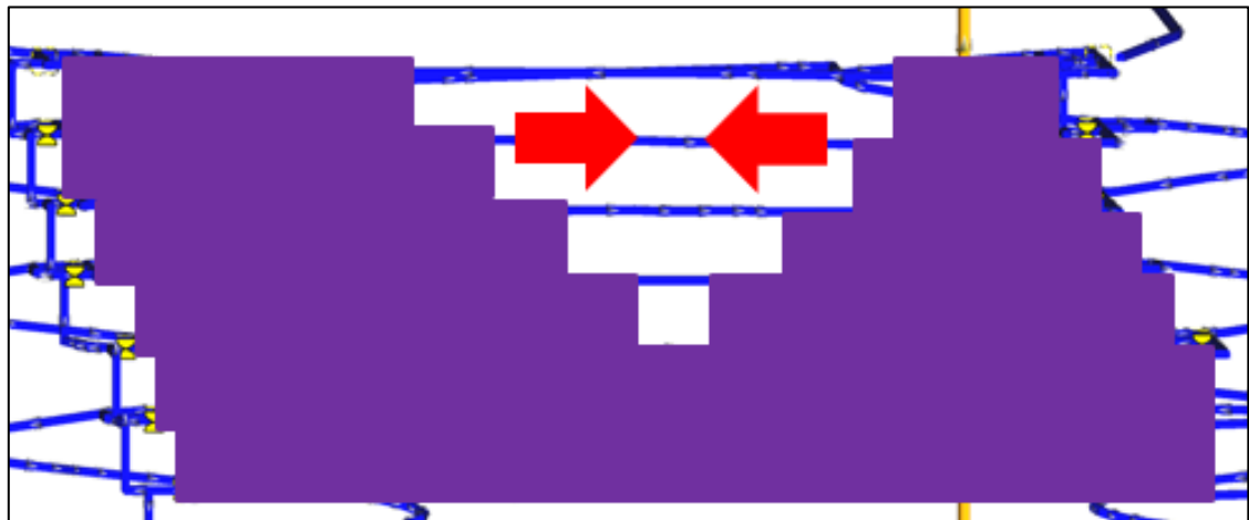
Figure 16-10 Current Outside-In Mining Sequence
