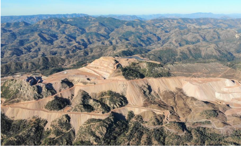
Pre-stripping open pit
