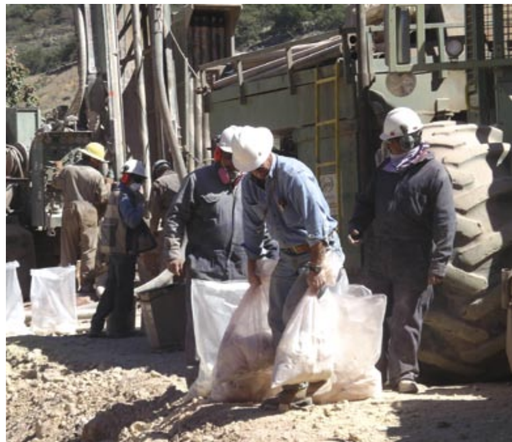
Drill cuttings are collected at the El Salto zone for delivery to the assay labs in Hermosillo, Mexico and Vancouver, British Columbia.
